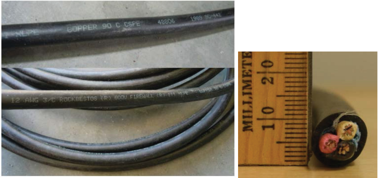
Figure 18. ROCKBESTOS® 600V FIREWALL® III XLPE cables and cross-section
