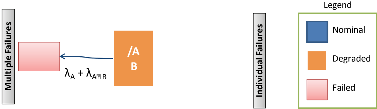
Figure B-2. Illustration of the degraded and failure states of a two-train system when EDG B is failed.
