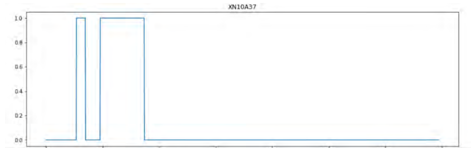
Figure 2. An example of an alarm signal that was created using the process events where a value of 0 represents the alarm off and a value of 1 represents the alarm on.
