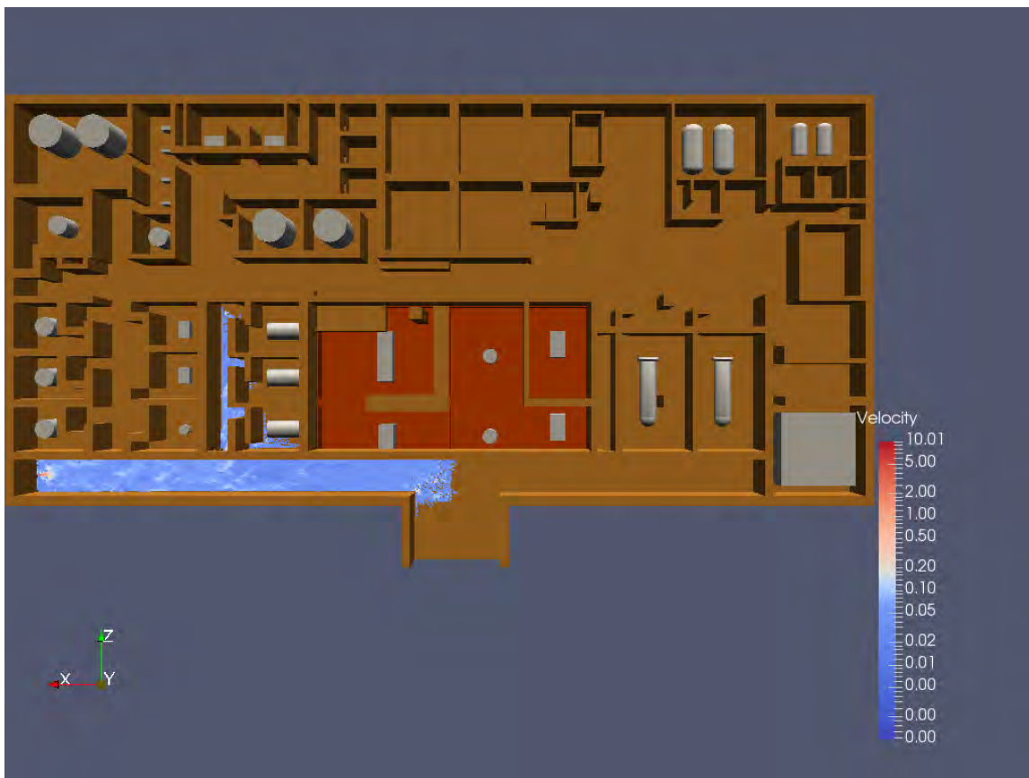
Figure 6-12. 3-D simulation – Auxiliary Building Underground Level 1.
