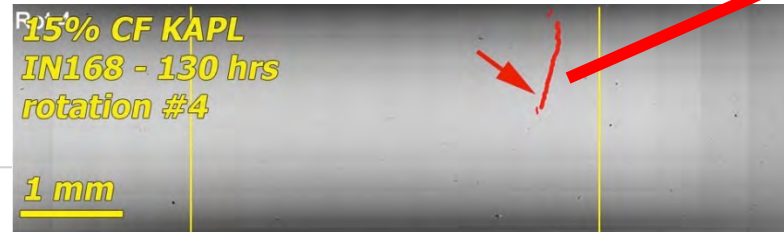
130 hours exposure (after DCPD initiation)
