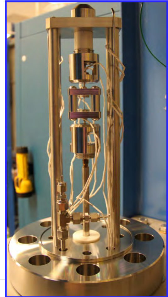
PNNL 2-3 Specimen SCC Initiation System
