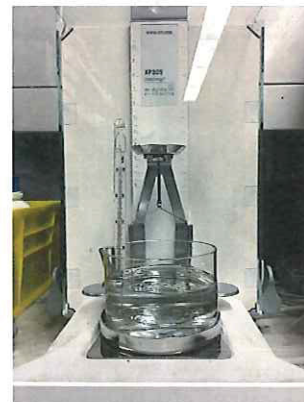
Fig. 8. Setup utilized in Archimedes density measurement.
