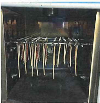
Fig. 6. Insulation sample arrangement utilized for accelerated thermal aging.
