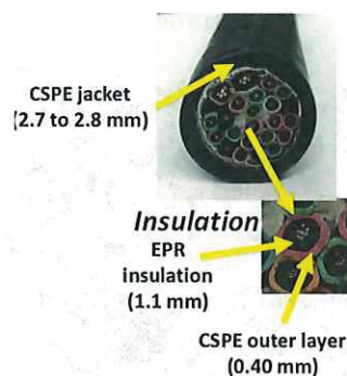
Fig. 5. Cross sections of insulated conductor from BIW cable that was harvested from existing NPP. Results that are related to this cable are referenced as BIW-A in this report.
