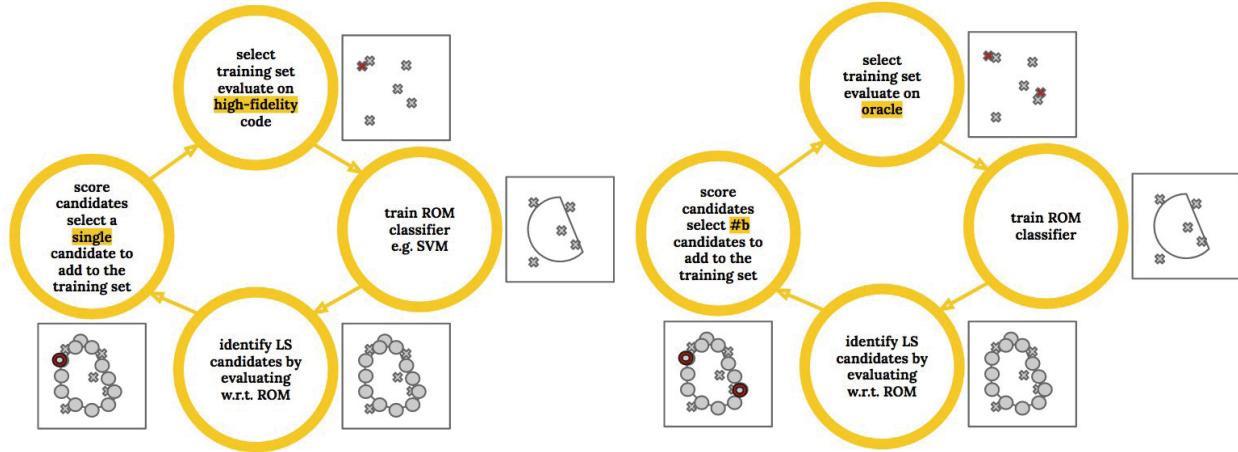
Figure 2. AS pipelines for RS search: serial mode (left) and batch mode (right). Training points are marked by crosses, RS candidates are marked by circles with selected ones marked in red.
