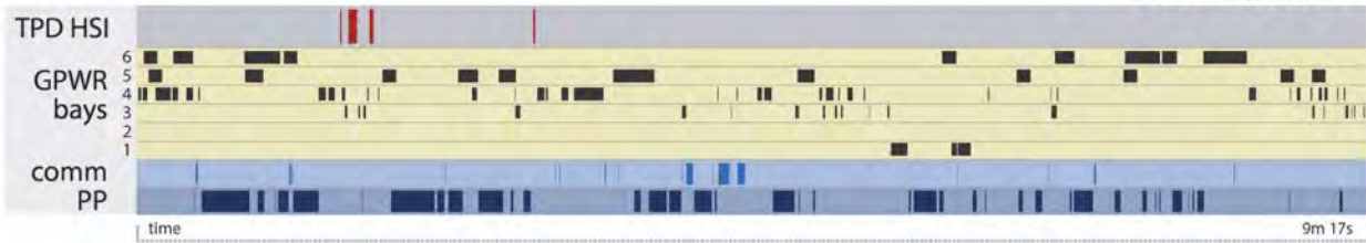
Figure D-9. Overall spatial and temporal distribution of fixations for Scenario 10: Load Rejection GPWR (governor valve failed close).
