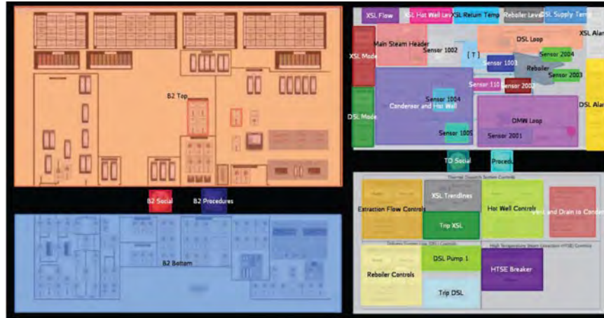
Figure 15. AOIs overlaid over the GPWR and TPD displays.
