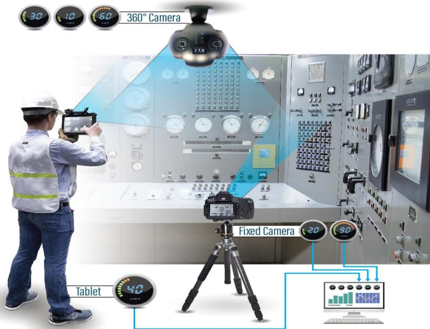
Figure 1. Automated gauge reading enables any camera to be used to log several gauges autonomously.
