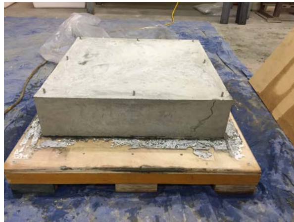
Figure 2. 2 ft × 2 ft × 6 in. dimension concrete slab (Vanderbilt University).
