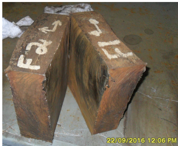
Figure 18. F1 and F2 blocks with orientations marked.
