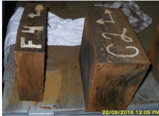
Figure 16. F4 and C2 blocks with orientations marked.
