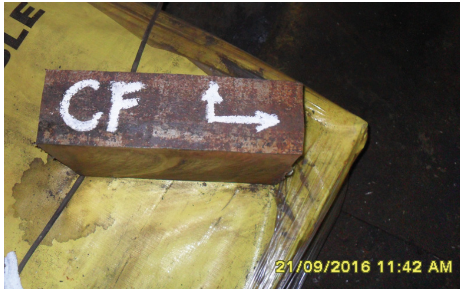
Figure 14. CF block with orientation marked (Y axis is perpendicular to the beltline weld with the arrow pointing to the top of the segment and the X axis is parallel to the beltline weld with the arrow pointing to away from the high fluence edge).
