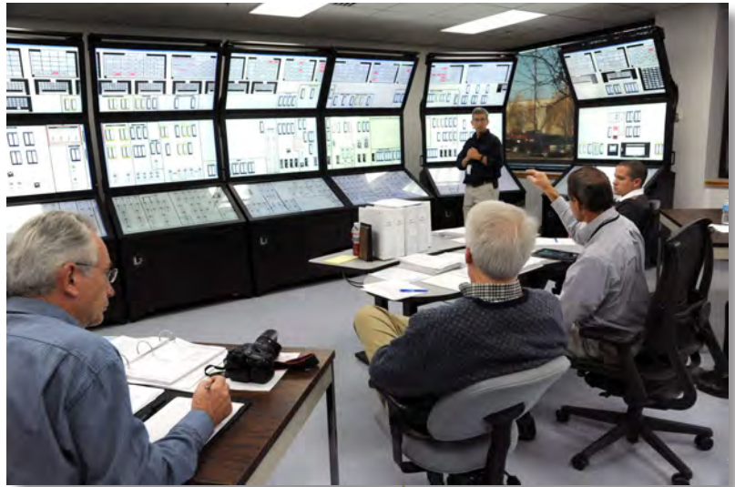
INL's Human Systems Simulation Laboratory (HSSL), capable of modeling a hybrid (analog and digital) nuclear power plant control room.
