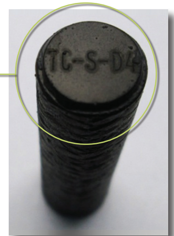
The cylindrical SiC-SiC composite tubes demonstrating General Atomics' successful joint fabrication
