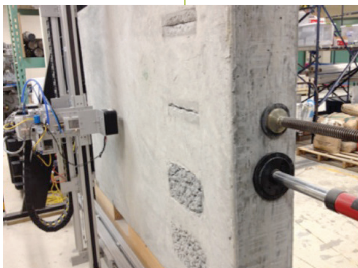
Ground penetrating radar scans and ultrasonic scans of concrete samples were performed at the University of Florida
