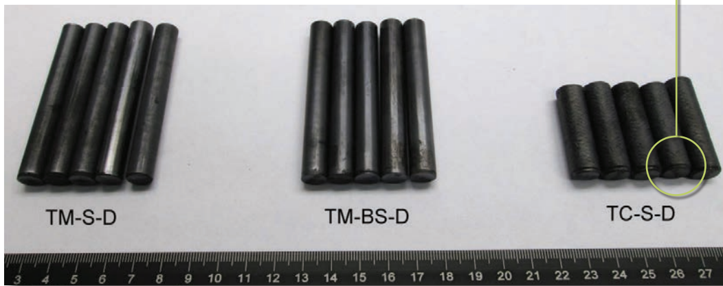
The cylindrical SiC-SiC composite tubes demonstrating General Atomics' successful joint fabrication
