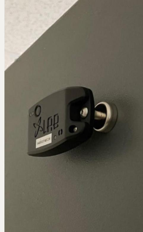
Ambient Temperature and Vibration Sensor
