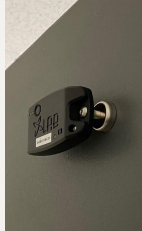
Ambient Temperature and Vibration Sensor
