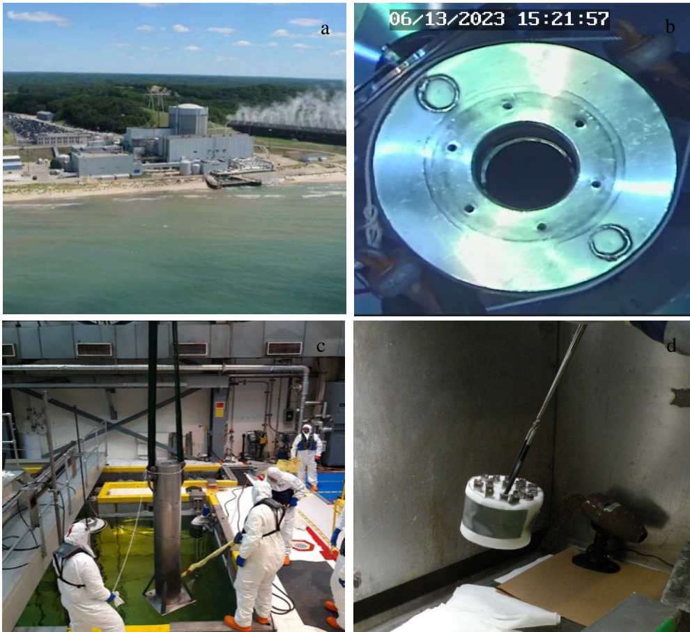
Figure 38. (a) View of Palisades nuclear power plant, (b) operation inside the spent nuclear fuel pool, (c) retrieve the cask loaded with the surveillance capsule, (d) specimen sorting and inventory inside the hot cell.
