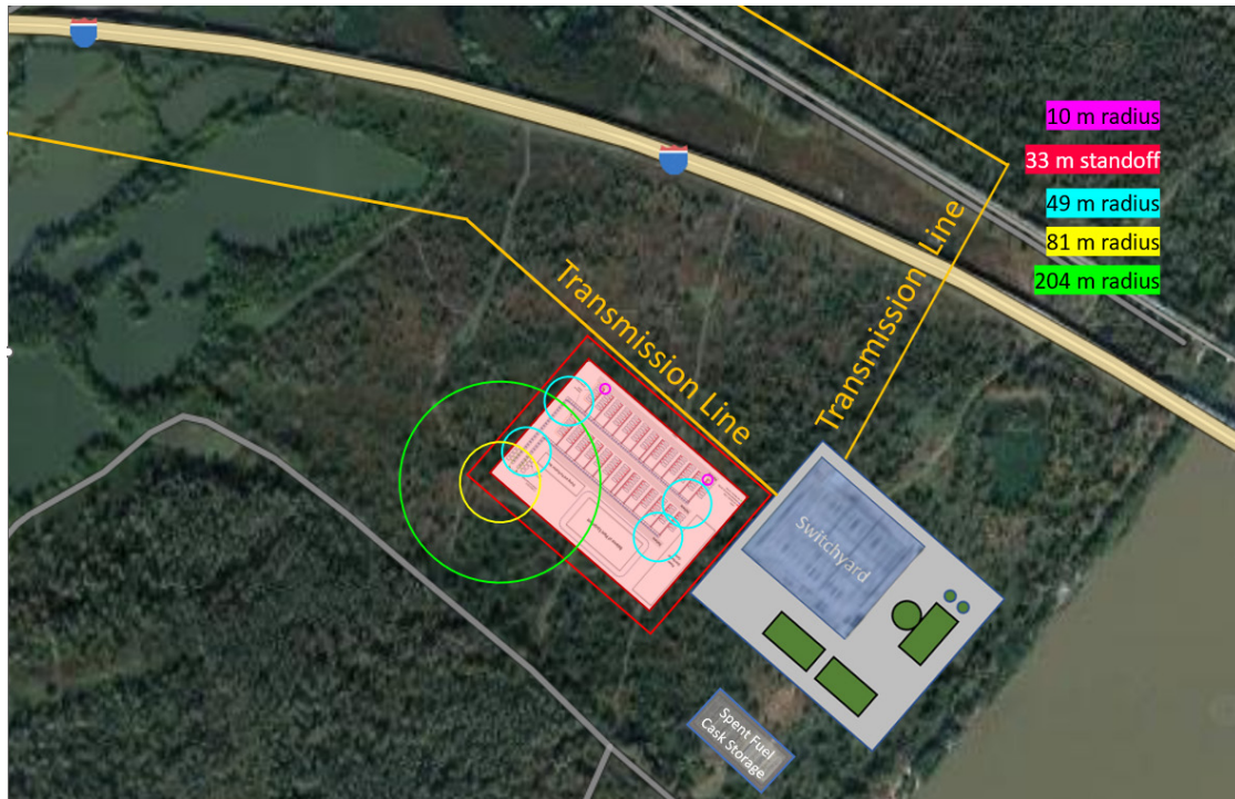
Figure 5. Illustrative safe boundaries surrounding hydrogen explosions for a 500 MWe electrolysis plant connected to a nuclear power plant.
