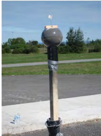
Figure 2-3. Experimental setup showing detonable explosive inside a glass bulb packed with iron powder [14].
