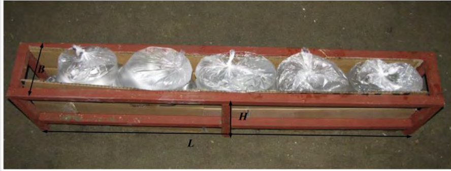
Figure 2-11. Top-down photo of water wall used in experiments conducted by Chen et. al. [32].
