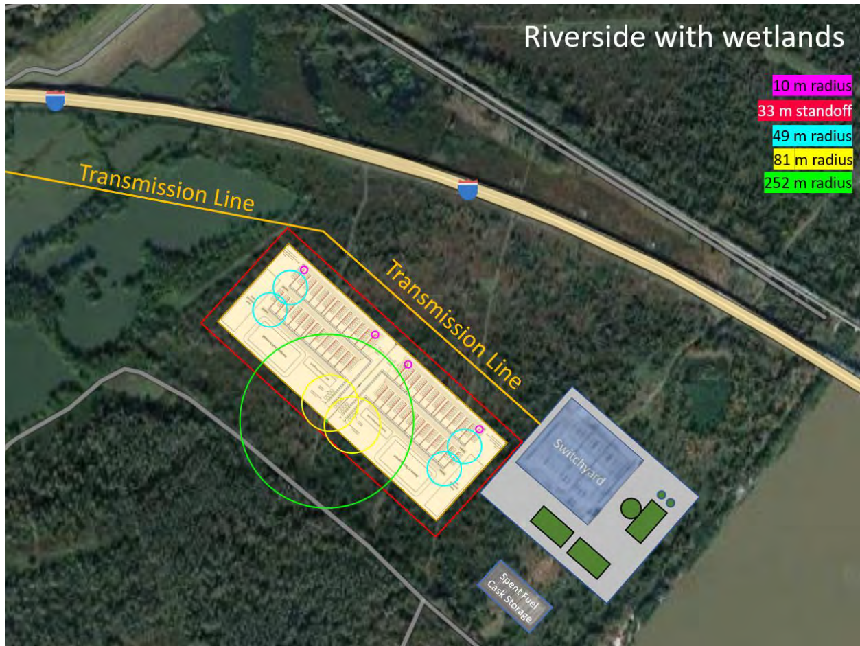
Figure 6-22. NRC RG-1.91 [11] Analysis for a 1000 MW nom HTEF of Site 1, “Riverside with wetlands.”
