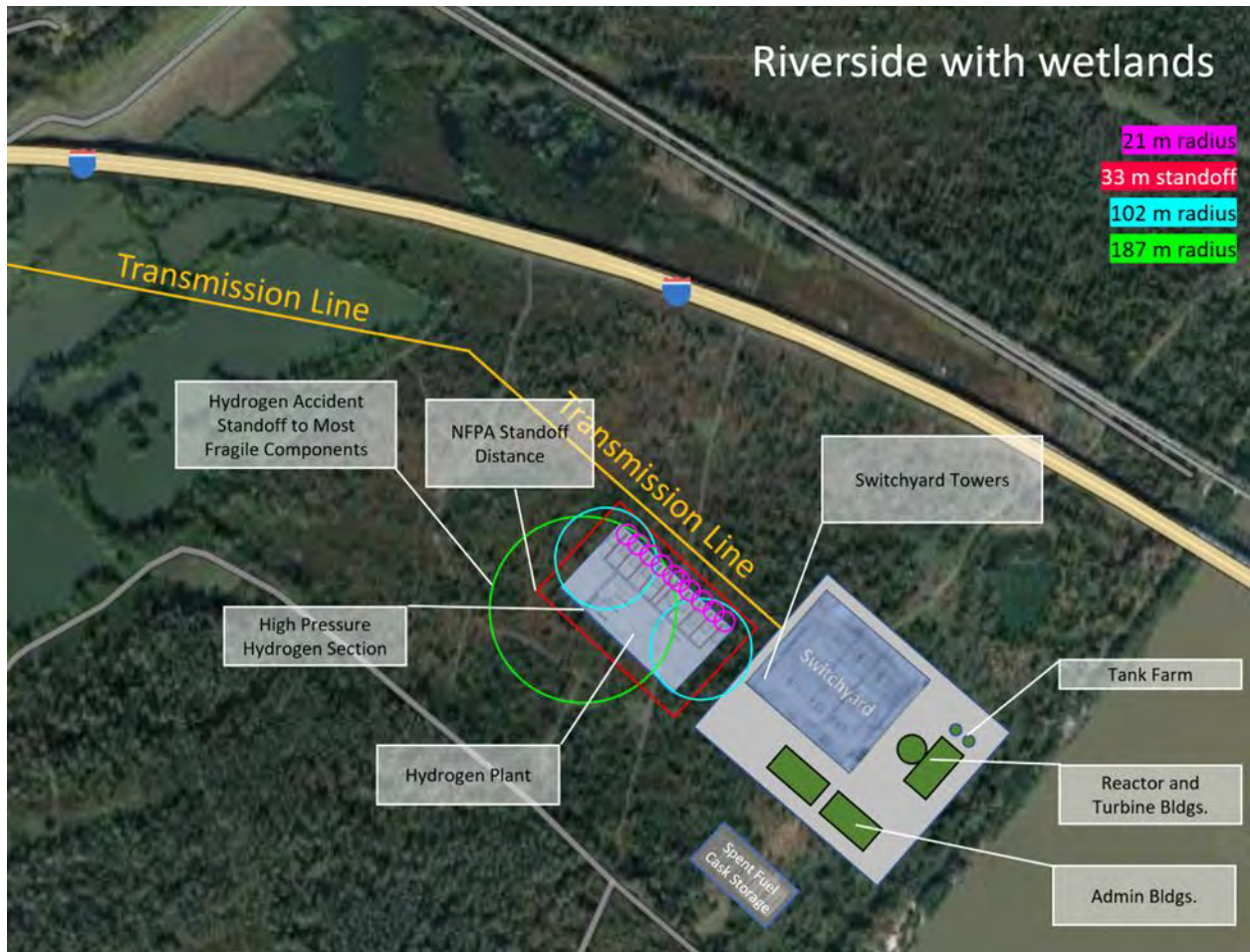
Figure 6-6. Bauwens Analysis for a 100 MW nom HTEF of Site 1, "Riverside with wetlands."
