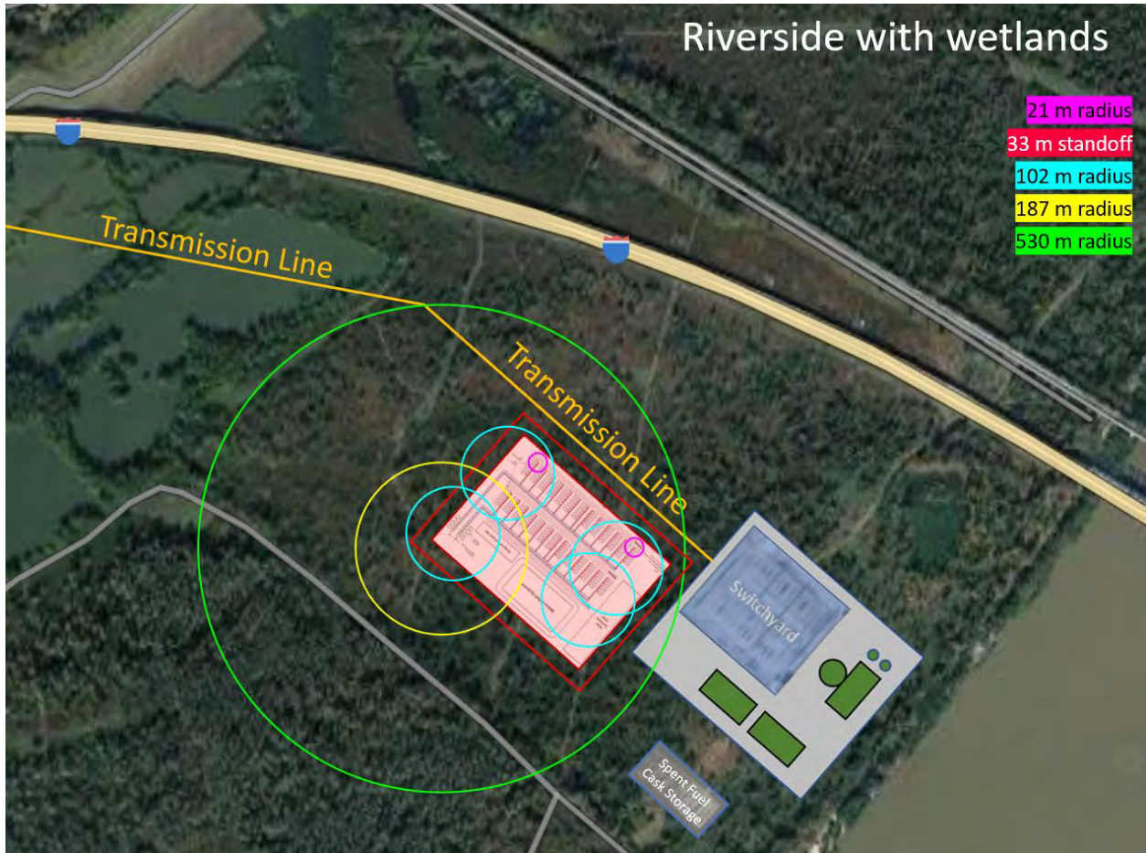
Figure 6-13. Bauwens Analysis for a 500 MW nom HTEF of Site 1, “Riverside with wetlands.”
