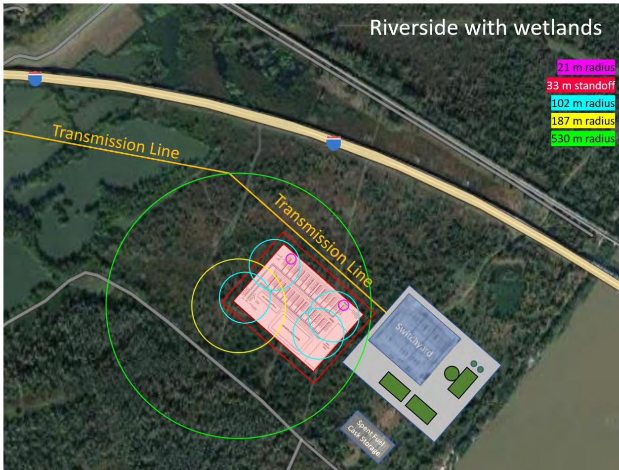
Figure 6-14. NRC RG-1.91 [11] Analysis for a 500 MW nom HTEF of Site 1, “Riverside with wetlands.”
