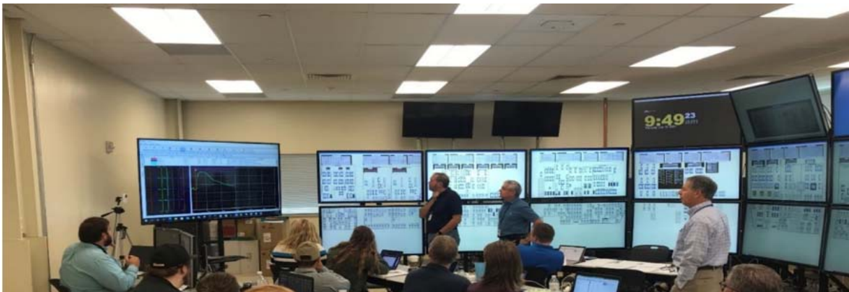
Figure 4. Human Systems Simulator Laboratory (HSSL) with virtual touch screens used to reproduce analog control panels to support TPD scenarios.
