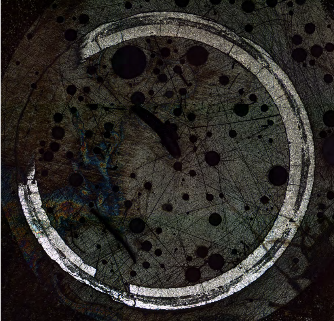
Figure 13. Clad ring sample about 1" from bottom. Difficulties were encountered in the preparation of this mount; however, some detail about the structure of the clad can be gleaned. Because of the poor nature of this mount, no information about the cracking is certain since the cracks may have occurred during the preparation; however, the clad was in poor condition prior to mounting so it is likely that some physical damage occurred during irradiation.
