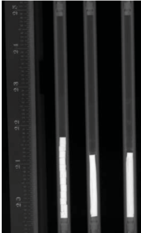
Figure 34. A neutron radiograph of irradiated fuel test specimens.
