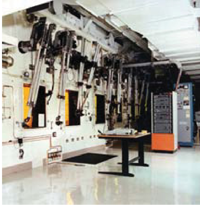
Figure 36. Work area in the ORNL Irradiated Materials Examination and Testing (IMET) facility facing the examination cells, showing manipulator controls for the remote handling of highly irradiated materials.
