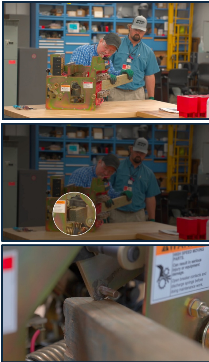
Figure 6. Pole shaft overtoggle test from the CBT video screenshot (left), pole shaft overtoggle test from the PowerPoint slides (right).
