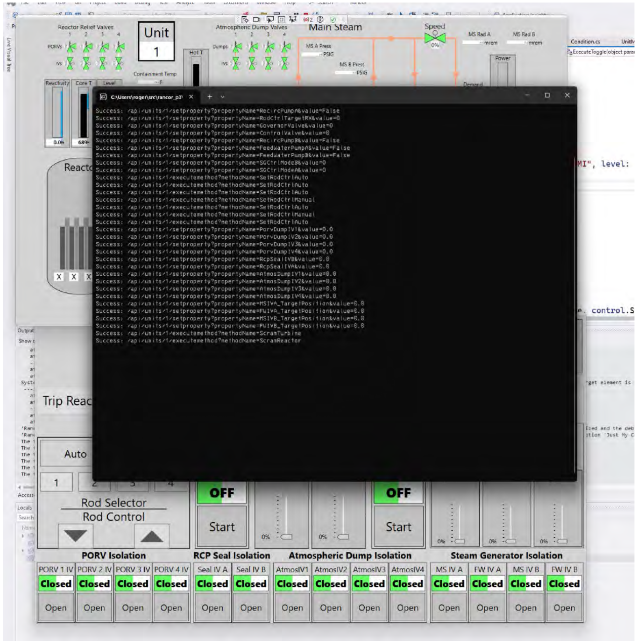
Figure 41. Rancor HSI running in client mode with the client is executing actions through the API
