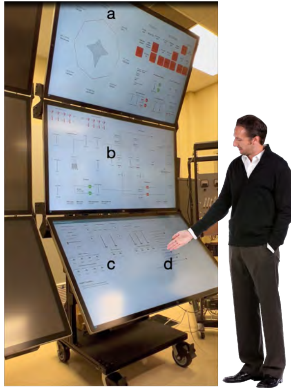
Figure 11. Rancor simulator displayed on a virtual bay supporting touch interaction with four distinct displays including overview (a), piping and instrumentation diagram (b), controls (c), and digital procedures (d)
