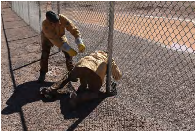
Figure 7. 8-in wire cutter and 36-in bolt cutter hand mechanical breach tests.
