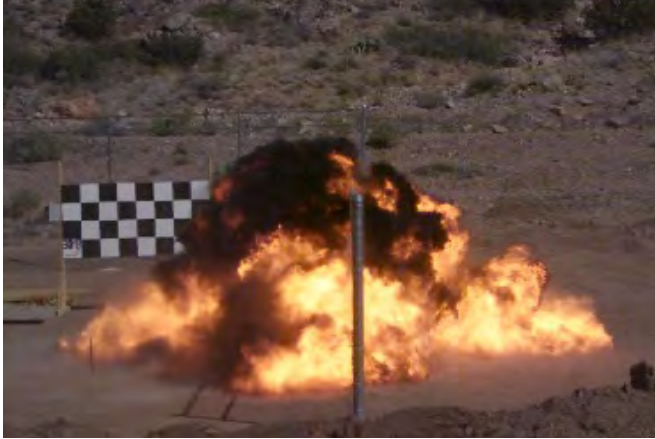
Figure 5. C-4 Charge explosive detonation fireball.
