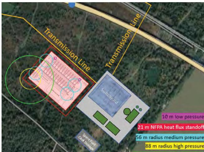
Figure 11. Safe standoff distances from a nuclear power plant to a HTEF.
