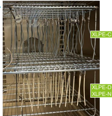
Hang the insulation straws on a rack for thermal aging
