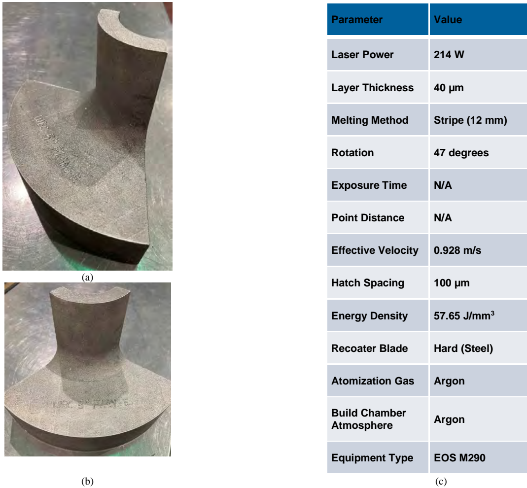
Figure 4 AM 316L flange produced by WEC and used to generate mechanical property data in air for the ASME code case # 20-254 [12] was received from EPRI.
