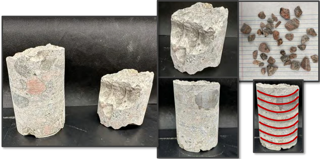
Figure 1. Unirradiated concrete cores from Ringhals Nuclear Power Plant. The smaller core was used to extract aggregates, and the taller core was sliced for analysis after running an XCT scan.
