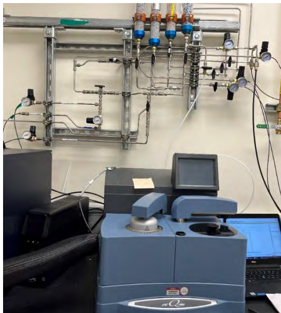
Figure 11. Differential scanning calorimeter for Oxidation Induction Time testing.
