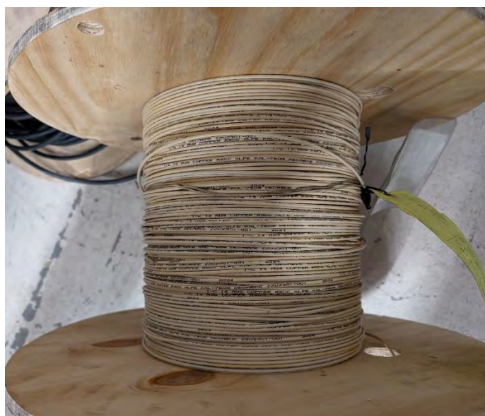
Figure 3. XLPE-dBDE cable insulation on a wooden spool.
