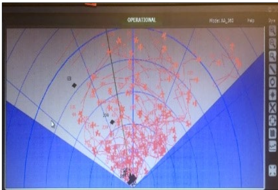
Figure E 1. Nuisance alarms generated during a light rain shower
