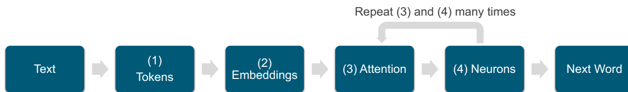
Figure 3. A basic flowchart of an LLM during the word generation process.
