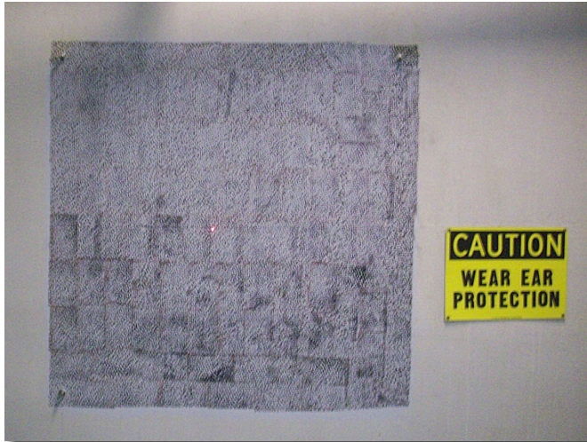
Figure 3. Speckled pattern applied to the upper containment location.
