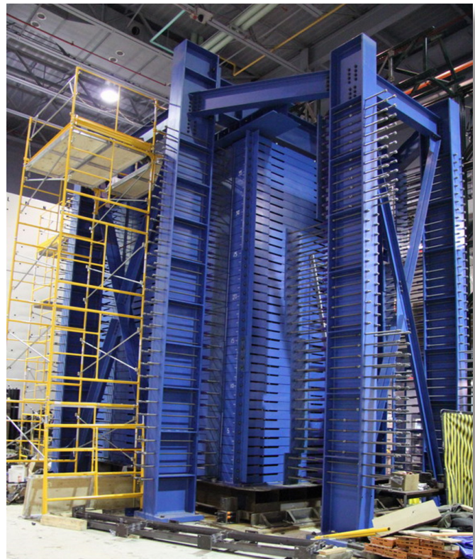
Figure 3. University at Buffalo's geotechnical laminar box.
